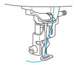
➤ The upper threading is finished. Now that the upper threading and the lower threading are finished, you are ready to start embroidering.
